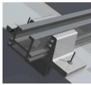
Figure 67: Inserting blind rivets
