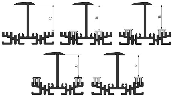
Figure 155: possible module frame heights
