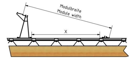
Figure 81: Distance AeroFix 15-S supports
