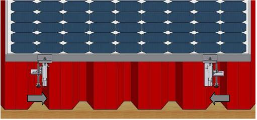
Figure 53: Mounted hanger bolt with "universal connector"
