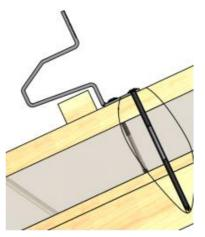
Figure 36: Inserting flat head screws
