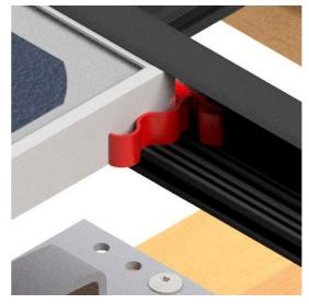
Figure 161: Insert spacer
