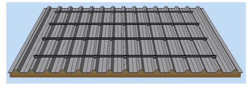
Figure 65: Mount carrier rail
