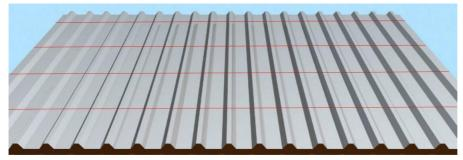
Figure 58: Marking fixing points
