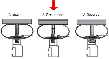
Figure 124: Inserting middle clamps G3
