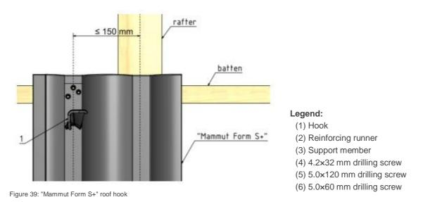
Specify the roof hook position so that you do not exceed a distance of 150 mm between fastener element (1) and the centre of the rafter.
