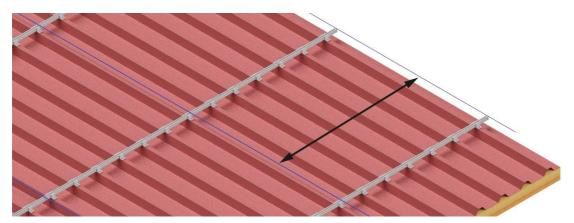
Figure 78: Mark the position of the Bottom Support in the grid spacing
