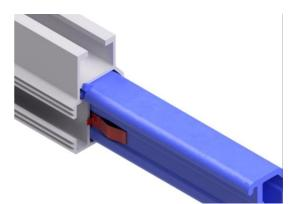
Figure 120: Insert butt connector (blue) and leaf spring for potential equalization (red) into the profile
