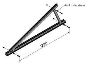
Figure 135: Assembling Delta supports at the base rails
