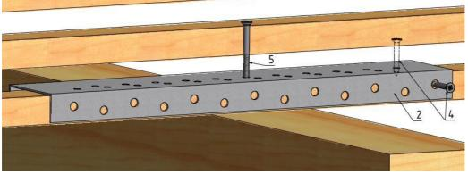
Figure 40: Fastening the batten rail
