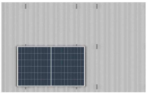
Figure 111 Aligning PV modules
