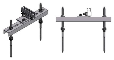
Figure 56: Mounting plate Duo with universal connector
