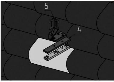
Figure 48: Roof hook fixing
