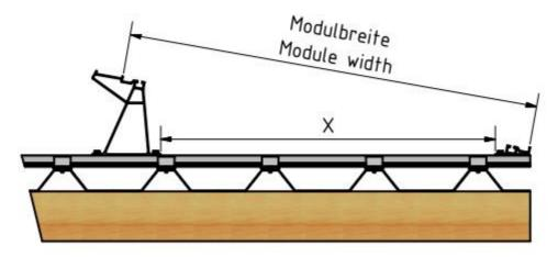
Figure 82: Distance AeroFix 10-S supports
