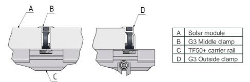
Figure 123: Assembled clamps (sectional view)
