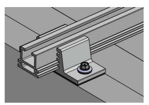
Figure 101: Apply the screw
