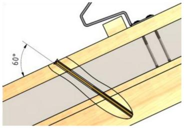
Figure 38: Inserting countersunk screws to absorb sliding forces
