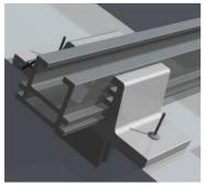
Figure 99: Inserting blind rivets
