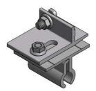
Use "Kalzip® clamps" to fasten the system on so-called Kalzip® roofs. The clamps are distributed vertically according to the number of cross girders. As a rule, fit one standing seam to each clamp. On each side the carrier rail must protrude by a maximum of 0.4 m.
