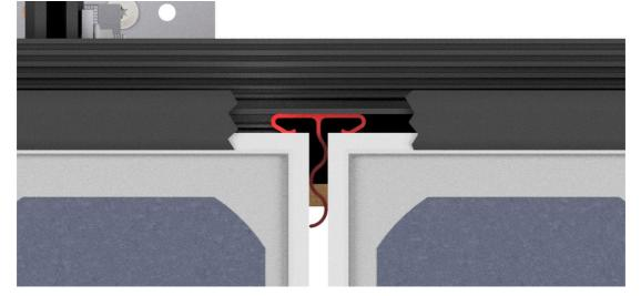
Figure 162: Mounted spacer
