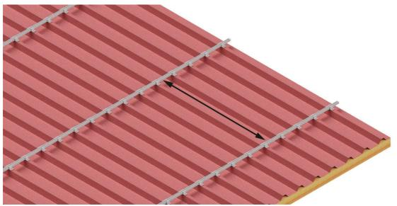
Figure 77: Gap = Module length + 20 mm
