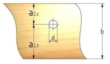
Figure 171: Defining the distance to the edge of rafters
