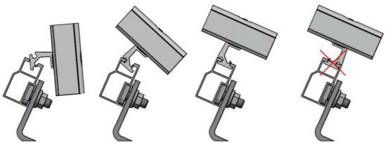
Figure 125: Inserting middle clamps G4
