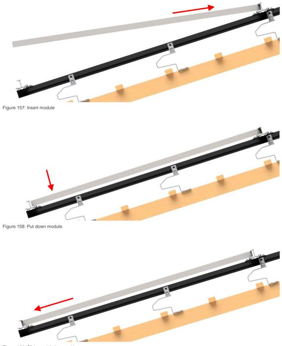
Figure 159: Slide module into position
