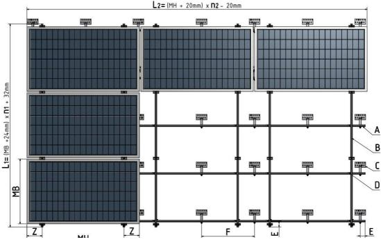
Figure 130: Roof hook connecting rails and carrier rails as a unit
