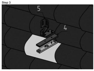
Figure 47: Cover cap and roof hook
