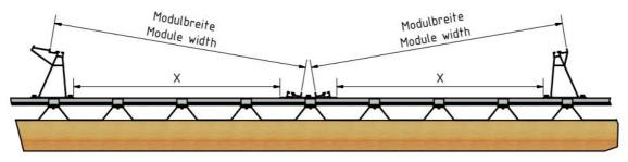
Figure 83: Distance AeroFix 10-EW supports
