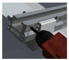
Figure 72: Drilling transverse securing clamps
