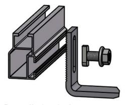
Figure 116: Carrier rail, fitted
