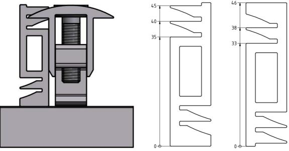
Figure 126: EC adapter with middle clamp G4
