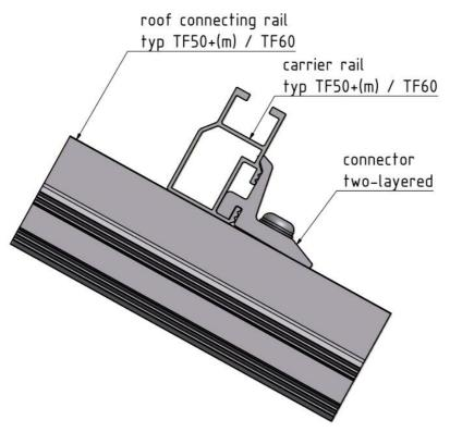
Figure 131: Cross section of a two-layer system structure
