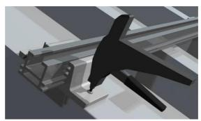
Figure 100: Riveting using a standard rivet head
