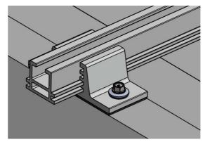
Figure 69: Apply the screw
