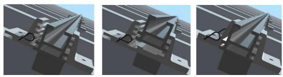
Figure 62: Insert the carrier rail
